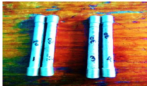
Fig. 1: Samples for tensile test
